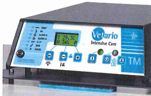
Figure 5: A digital read-out is an extremely useful feature to have on an incubator
