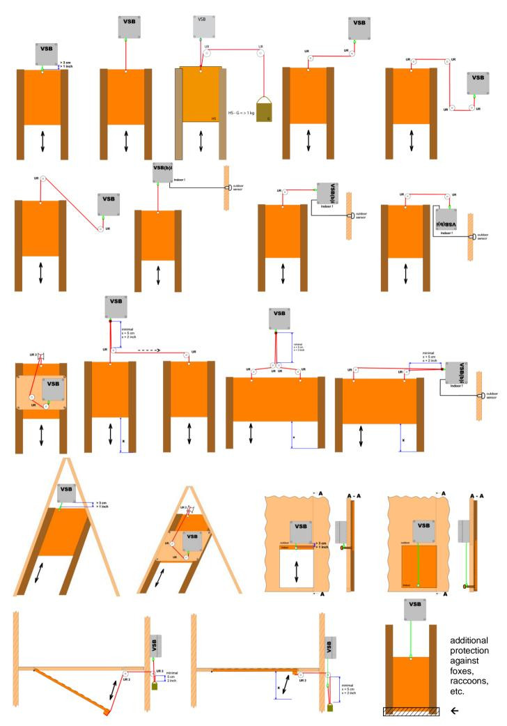
**green cord:** *internal cord of the VSB*, do not make any changes! Do not pull out the cord by yourself! **red line:** external cord, extension cord, use if VSB is not mounted directly above the slide. Cord may be guided over pulleys > see description above
