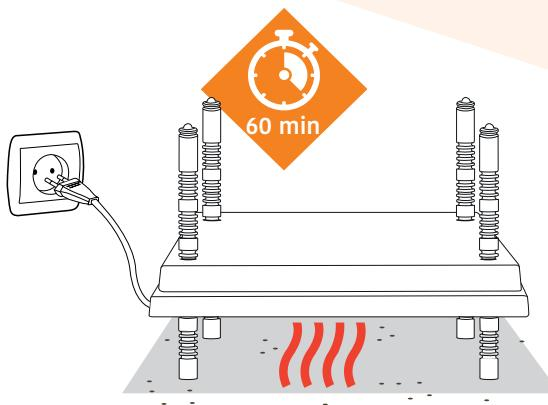
When all legs have been mounted to the right height, the heating plate can be placed into the rearing unit. Connect the plug to the power supply and you will see the red LED indication lighting up. After approximately 60 minutes the maximum temperature will be reached, and the chicks can be released near the heating plate.
