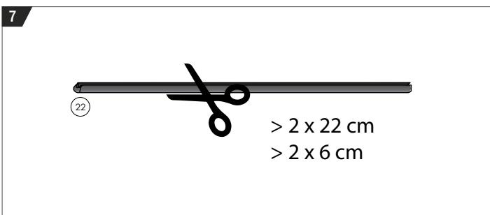
**EN** Cut the rubber band (22) into 4 pieces using the lengths beside>>
