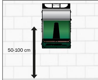
**EN** Place the laying nest at a dry and draft-free place, on the wall at 50-100 cm height. Make sure the nest is 100% level.
