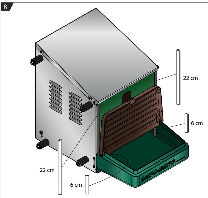
**EN** Attach the rubber band on the laying nest by sliding them in place.
