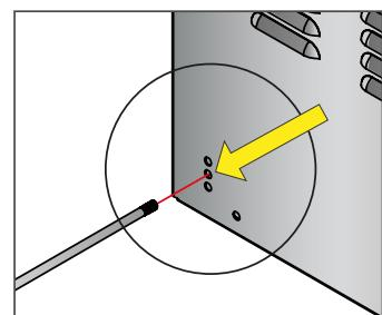
**EN** The bottom plate with the brown nest pad can be set at three different angles where the eggs will naturally roll into the collecting tray. There are three options, but we advise to use the middle hole.
