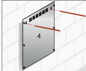
**EN** Before starting with the assembly, use the metal back side (4) of the laying nest as a template to mark the right location for the screw holes on the wall.
